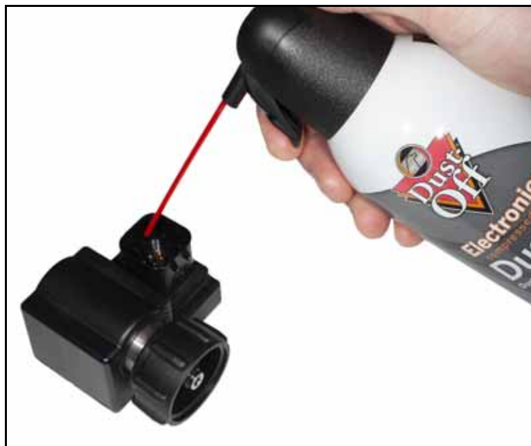
FIGURE 3. Compressed Air Used to Dry Connector
